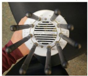
D. Below is an example of an AT7 positioned for calibration. The best way to calibrate with the AT7 is to lay it flat, with the W0 and W3 label sticking up on the 2.4/5 side, which corresponds to both 2.4G and 5G W0 antennas sticking up. The rest of the antennas can be facing as down as possible and away from the two pointing up.
