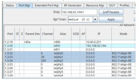
3. Then click **Sniff Packets** and the LANforge server will create multiple monitor interfaces, then one (or more) Wireshark instances will appear sniffing traffic.
