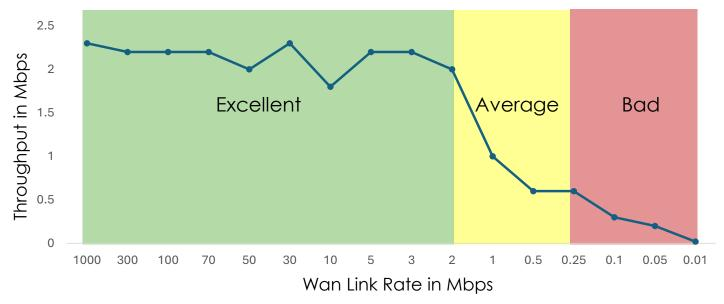
The DUT transmitted the data without packet drops till 2Mbps and the video log at monitoring device is excellent without any buffers. As the link rate at WAN is restricted between 2Mbps and 250Kbps, there is noticeable buffers. As the link rate is further restricted beyond 250Kbps, the video is unusable with complete buffering
