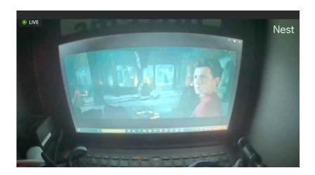
Noticeable video buffering is observed when channel utilization is over 90%. Video play is good till 80% channel utilization.
