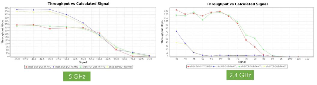
UDP/TCP, Upstream/Downstream throughput is calculated by increasing attenuation between the AP and the tester in 5dB steps programmatically.
