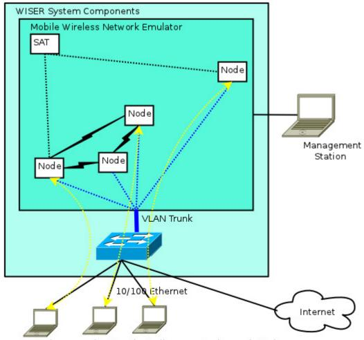
End-user applications logically connected to each Node in the emulated network. Each physical port on the switch is connected directly to an individual node through use of 802.1Q VLANs.
