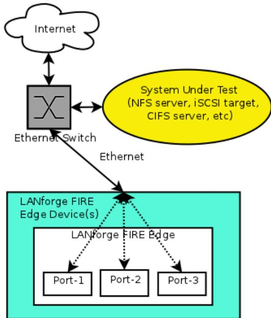
LANforge FIRE supports multiple Ethernet interfaces. To the System Under Test, it appears as if each virtual and physical interface is a separate PC or network appliance generating independent stateful traffic streams.
