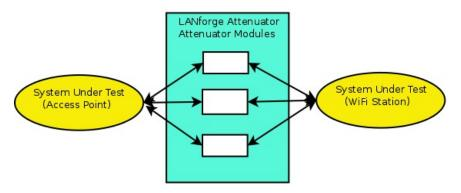
The LANforge attenuator sits between two RF systems, often a WiFi AP on one side and WiFi Station on the other. The attenuator and WiFi stations are connected by shielded SMA-Male cables. Adjust the attenuation as desired using either the attenuator knobs or use software to adjust the values over the USB-Serial connection.
