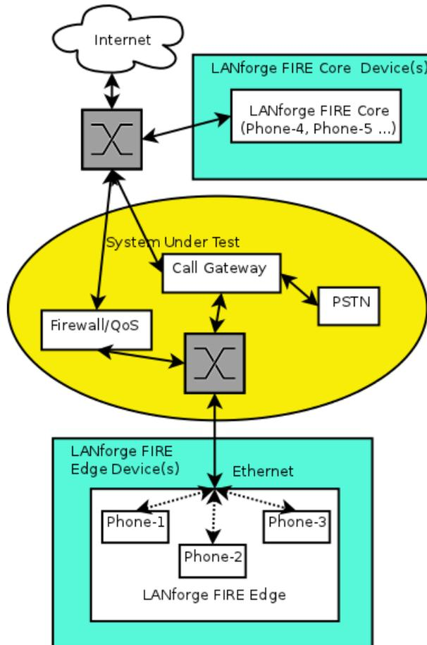
LANforge FIRE supports multiple Ethernet and Virtual interfaces. To the System Under Test, it appears as if each interface is a separate PC or network appliance generating independent stateful traffic streams.
