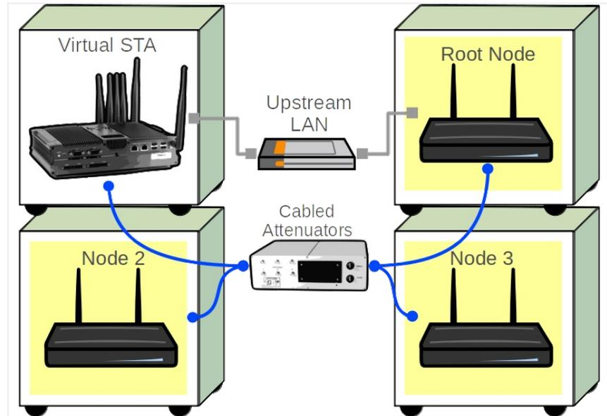
1. Configure Chamber View for Mesh and Similar Tests.
