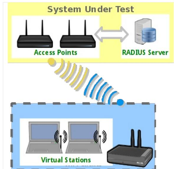
1. Configure stations to connect to an AP configured for HotSpot 2.0.
