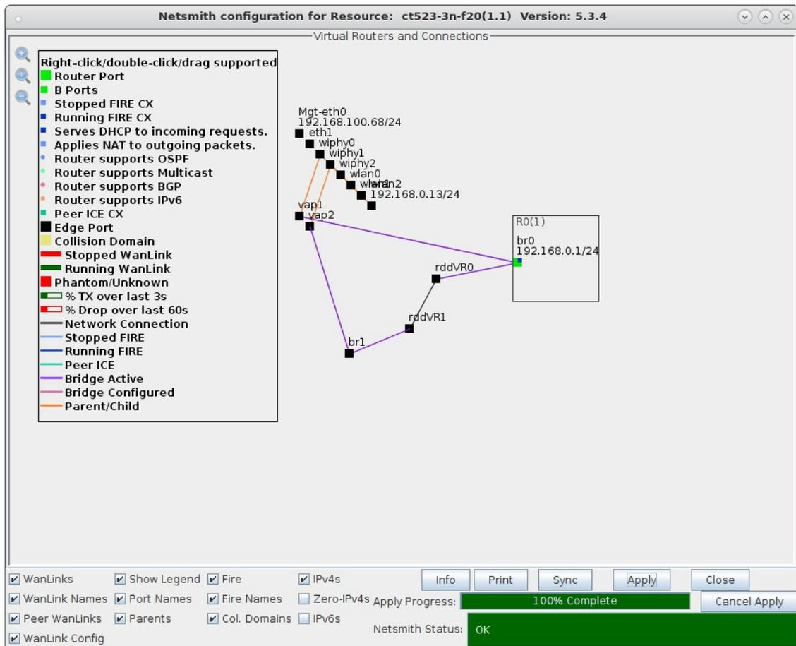
6. Connect clients and force them to roam from vap to vap. This can be accomplished with a `wpa_cli` command for one or two clients or the Mobility Plugin Script for many clients. If the system under test is not able to force a roam, a variable attenuator on each vap radio may help induce a client to roam as the signal strength from vap to vap is varied.
