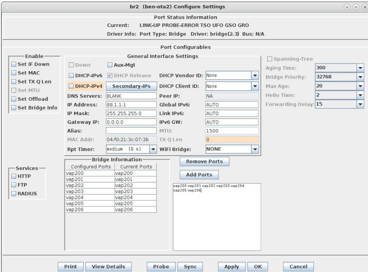
4. Create a virtual router in Netsmith and add br2, and optionally a wired port (eth1) to the router. Double-click the br2 port and configure DHCP to match its IP address. When complete, Netsmith should look something like this:
