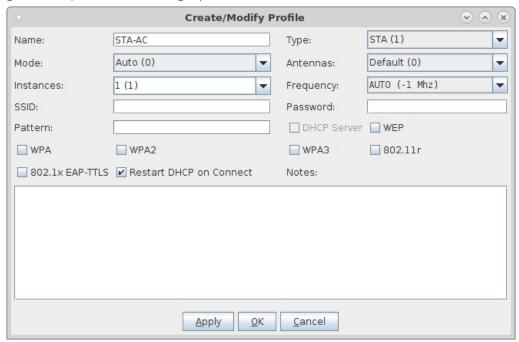
F. Configure a Chamber View Scenario and add the STA profile (mapped to desired wiphyX radio and DUT). Add an upstream profile mapped to DUT LAN side (or possibly WAN side if that is more appropriate for your DUT). Please note that we will manually configure the station to connect to the second DUT as part of the test steps below.
