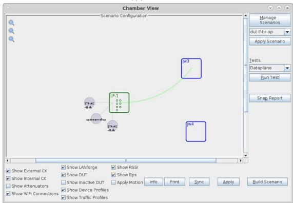
B. Select the **Dataplane** test and click **Run Test**. You should see the RX Sensitivity Test configuration window pop up. It will remember the last configuration for most fields. Select the DUT and WiFi station device, and select the combinations of traffic types you wish to send. Select the **Another Iteration** checkbox to allow comparison graphs.:
