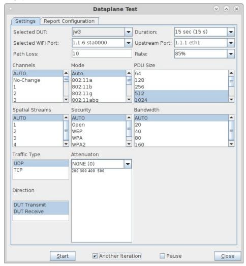
C. We have 4 total BSSIDs that we wish to test. The Scenario creation logic will have chosen one of the BSSIDs for the station, but we will need to override that for each of our comparison runs. Go to the Port-Mgr tab in the LANforge-GUI, double-click the station, and make sure that its SSID is correct. In case you are using different passwords you could change that at this time as well. When complete, click Apply. You can leave the window open as you will need it in future steps:
