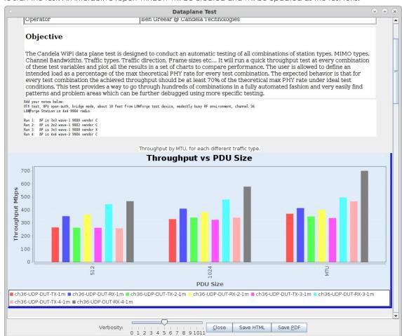
E. When the first comparison run is complete, a popup window will be shown, and the **Paused** checkbox will be selected. Select new BSSID by reconfiguring the station with a new BSSID, and when the reconfiguration is complete, un-select the Paused checkbox on the Dataplane test to do the next comparison run. Continue to run new comparisons in this manner until the full test is complete. When complete, unselect the **Another Iteration**, and then unselect 'Paused\* to have the test complete:
