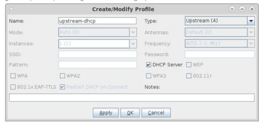
E. Configure an STA profile on the LANforge system.
