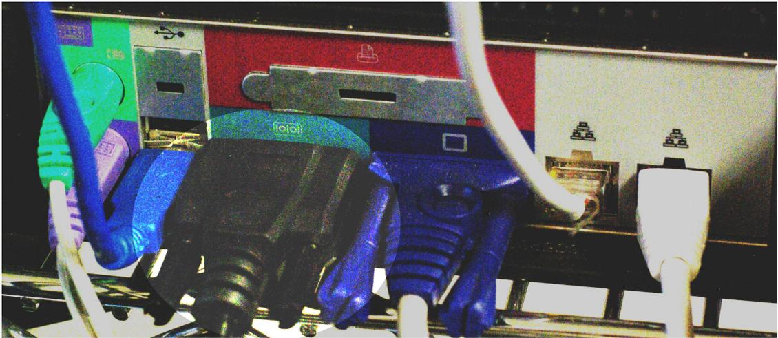
E. Other LANforge chassis models can have either RJ45 or DB9 serial ports.
