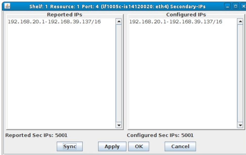
D. Make sure a second ethernet port on the LANforge is properly configured for the server-side of the network. In this case, we are using a network-emulator in bridge mode as device-under-test, so all IP addresses are on the same subnet.
