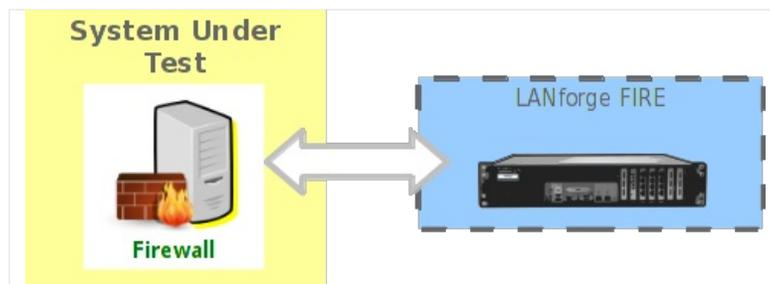
1. The **UDP Throughput** test will use a scripted Layer-3 connection to vary the rate and payload size to determine the bi-directional UDP throughput of the DUT across the scripted parameters.
