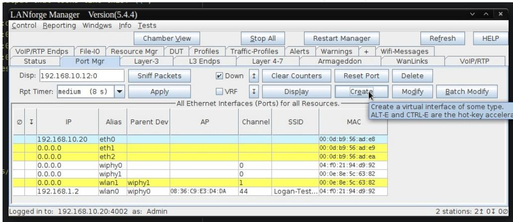
B. Next we will create the station, the default values can be used or a specific number for the station can be given:
