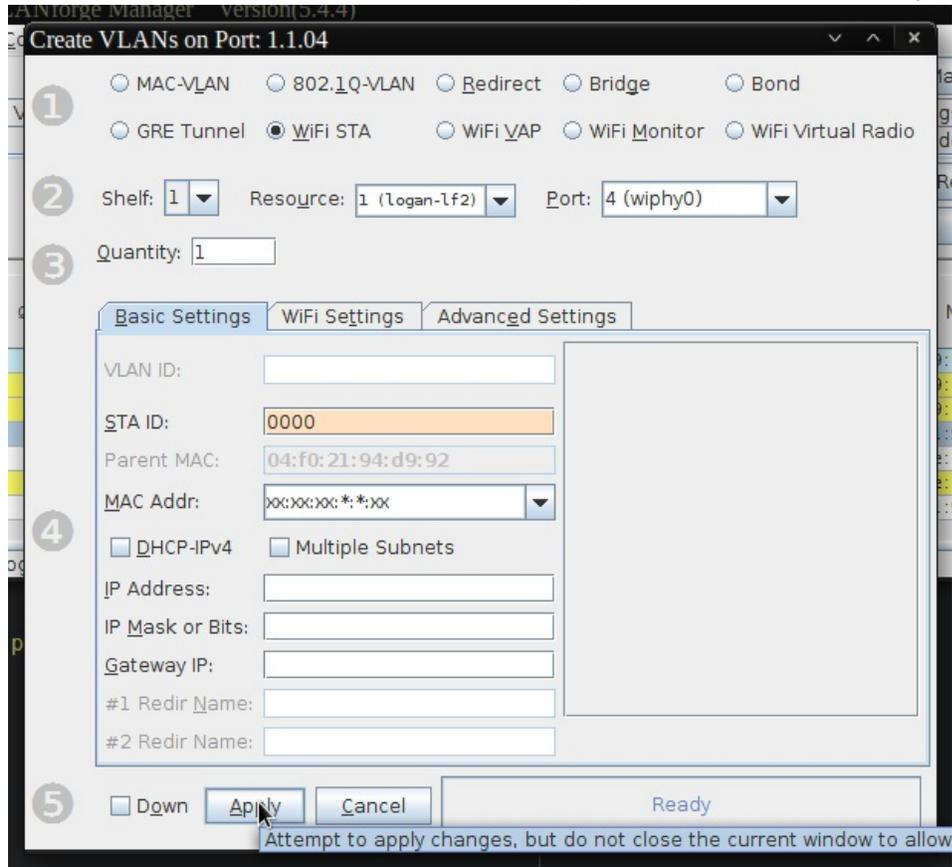
C. After creating the station, we will give the an SSID to connect to. (This doesn't have to be a real AP):
