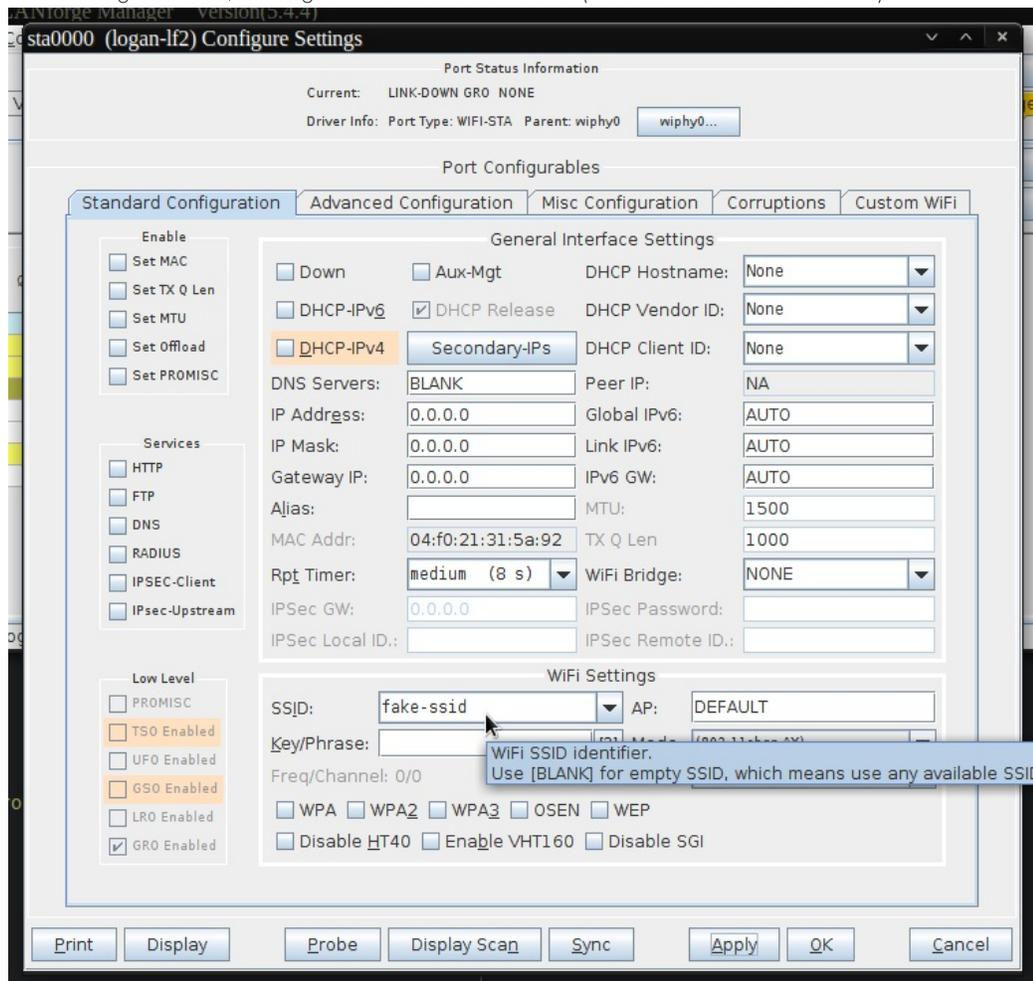
D. Clicking on Display Scan at the bottom of the station settings window will bring us to the Scan window:
