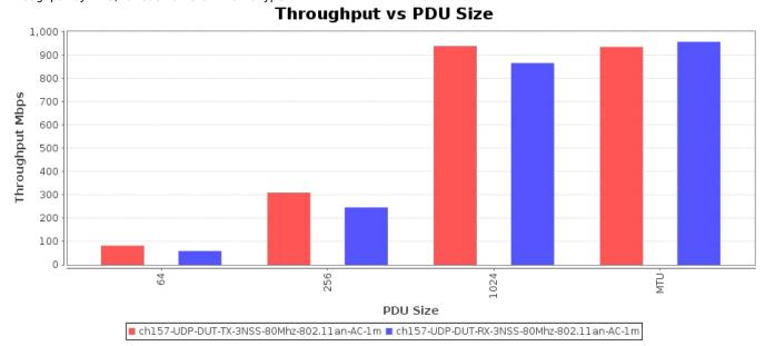
Pps throughput by MTU, for each different traffic type. The values are estimated packets-per-second over the DUT, but some protocols such as TCP make this difficult to know for certain, so the value is extrapolated.
