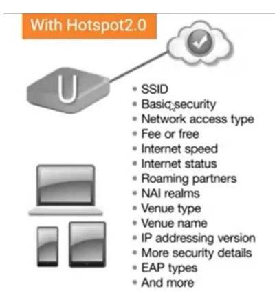
Hotspot 2.0, also known as Passpoint, is a set of standardized protocols developed by the Wi-Fi Alliance. In the beacon frame of a hotspot Access point, we have the details of the cellular providers and roaming partners it supports. Helping Wi-Fi offloading from cellular.
