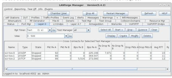
D. Here are the details of the endpoints. Notice each sent 99 pdus as requested with the --txpkts option.
