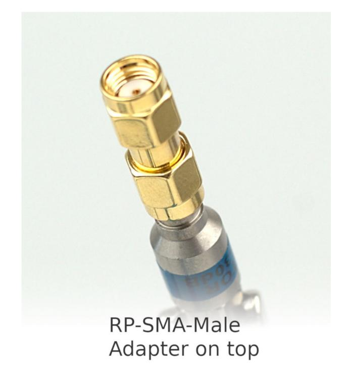
3. We see that the exposed end of the sma\_adapter is RP-SMA-Male. RP means Reverse Polarity.
