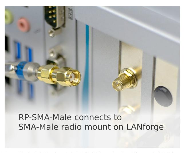
4. Connect the attached attenuator and adapter to the LANforge radio antenna. This exposes the SMA Male end of the attenuator. Your DUT might not have adequate space to mount a fixed attenuator to it, so we suggested connecting it to the LANforge.
