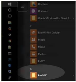
4. Double click the vnc icon and it will ask you for the IP address. You want to set the Encryption option to **off** because we presume you are connected directly to the LANforge.
