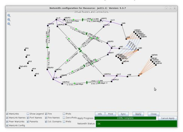
C. Create 5 connections between the rddD and rddF ports
