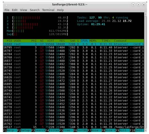
A. The majority of btserver processes with the same or similar values here represent the running File-IO endpoints. The RES (resident value) column represents the memory used by these File-IO endpoints. The current test uses an average of about 10,400 KiB or 10.6 MB per btserver process. These values should be monitored as the File-IO settings are adjusted.
