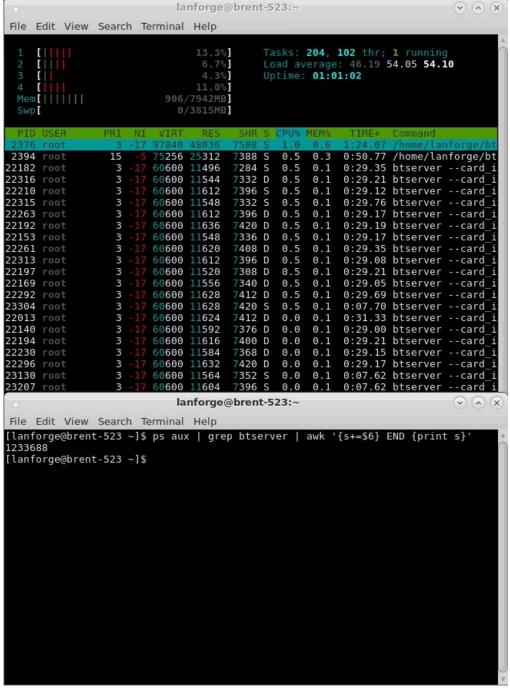
A. Changing the Min/Max RW sizes to 1MB increased the btserver memory use to about 11,600 KiB or 11.9 MB from 10,400 KiB or 10.6 MB. About a 1,200 KiB or 1.3 MB difference.
